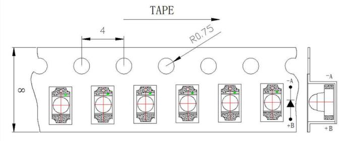
Note: Tolerance unless mentioned is ±0.1mm; Unit = mm
