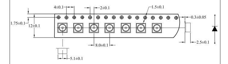
Note: Tolerance unless mentioned is ±0.1mm; Unit = mm
